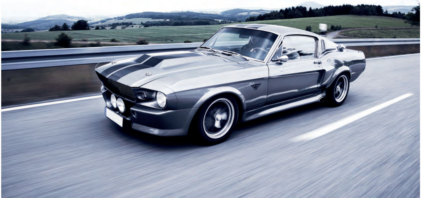
Ford Mustang Eleanor, Frame-Off-Restauration, Boss 5,0 V8 supercharged Motor, 500 PS
